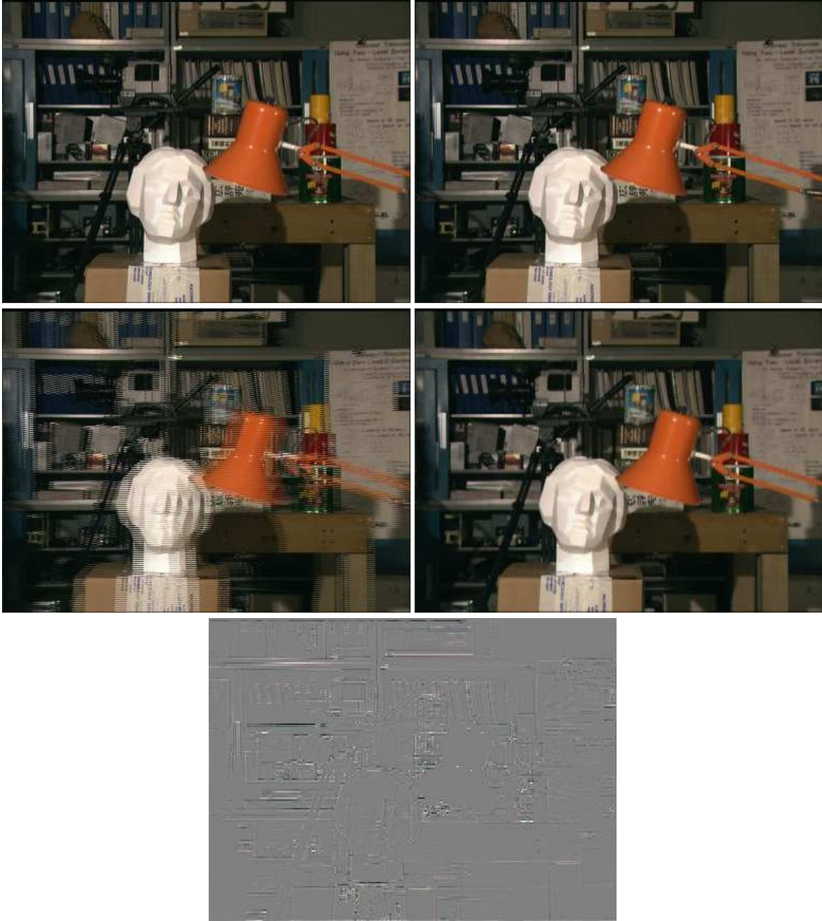
**Fig. 4** Test example for deinterlacing, *top left*: first frame, *top right*: second frame, *middle left*: interlaced data, *middle right*: result of applying the proposed PDE with initial data  $\mathbf{u}^{(0)}$ , *bottom left*: difference between  $\mathbf{u}_1$  and the deinterlaced result.
