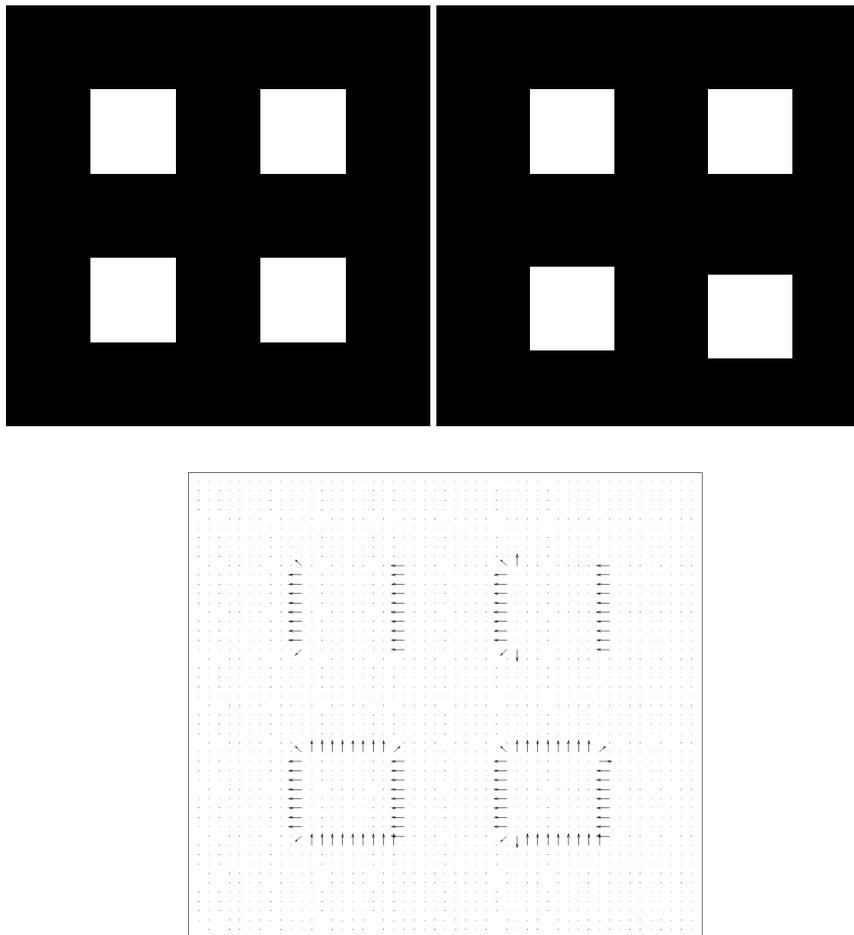
**Fig. 1** Test example for computing displacements via pseudo-inverse. Top left: Test image with four objects. Top right: image with shifted objects. The top objects are shifted to the right by one and two pixels, respectively. The bottom objects are shifted diagonally with a displacement of length  $\sqrt{2}$  and  $\sqrt{8}$ . Bottom: displacement calculated using the Moore–Penrose pseudo-inverse, see (5).
