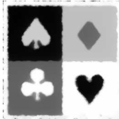
Figure 4: Resulting image after applying the BV-Filter with \alpha = .1, \tau = .01 and 10 iteration steps of the explicit scheme.
