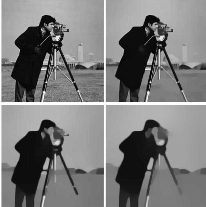
Figure 4: Original image (top left) and iteratively filtered images using p = 1 and \alpha = 0.1 (top right), \alpha = 0.5 (bottom left) and \alpha = 1 (bottom right), respectively.
